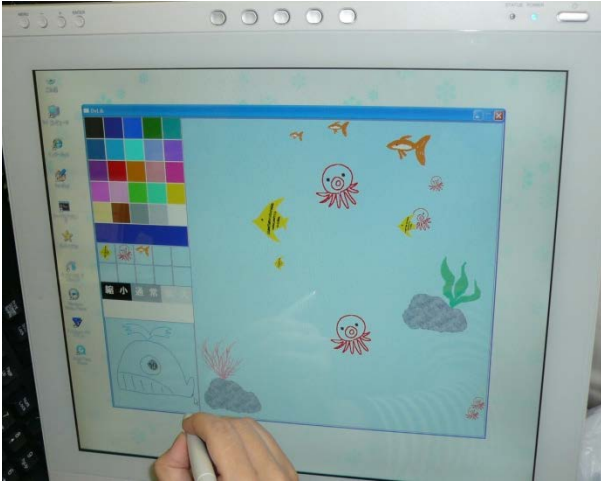
Fig.5 Users can draw any object on the screen by electronic pen and put it in "swim" field. Same objects gather and show the collective behaviors based on the proposed kinetics.
