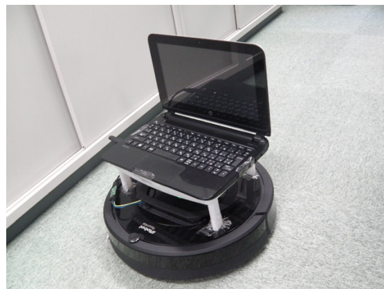
図 1: AcToR(Active Touch Communication Robot)
