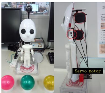
Fig. 2. Placement of the servo motor
