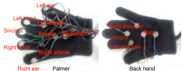
Fig. 2 Haptic glove equipped with 14 vibration motors, with each motor corresponding to one of the colony agent’s touch sensors
