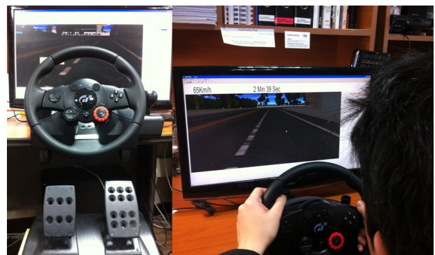
Figure 1. Experiments environment 3-Dim. Driving simulator and Logitech wheel joystick with 2 state pedals
